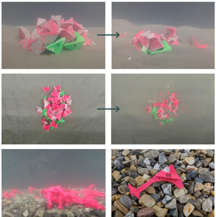
This experiment was executed in a flow flume, so there is only flow loading. In normal conditions, waves influence the bed as well. The flume produces a water flow in a single direction; in real conditions, the flow is not that stable and could vary. The tides change direction every six hours, meaning that the water flows in the opposite direction when this happens. This could not be tested in the flume.
