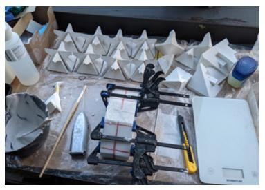
Figure 45: Casting of prototype in silicone mold.
