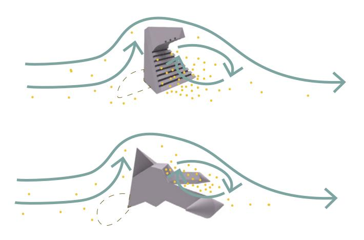
Figure 62: Sediment depostion mechanics.
