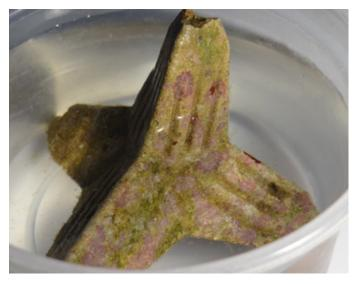
Figure 26: Biofilm on a concrete unit (photo: SECORE).
