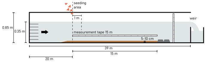
Figure 51: Setup for the flume.
